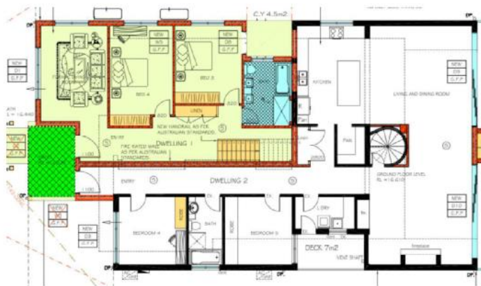
Figure 1. Reduction in the FSR of the ground floor level shown in green
