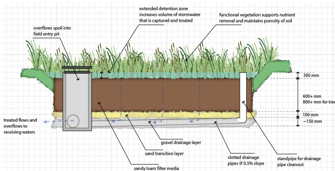
**Figure 1: Bioretention system typical arrangement (Water by Design 2009)**
