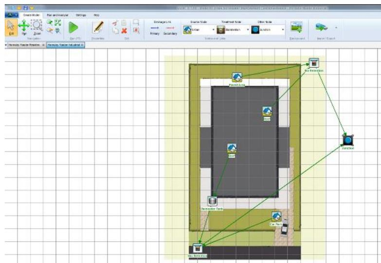
The roof and paved area draining the back of the property were treated in a bioretention system. The total area draining the back of the property is 685m<sup>2</sup> (roof 640m<sup>2</sup> and paved area 45m<sup>2</sup>). An approximate size of the bioretention system would be 1.5% of the area, or 10m<sup>2</sup>. A bioretention of 15m<sup>2</sup> was modelled and found to meet the pollution loads from the catchment.
