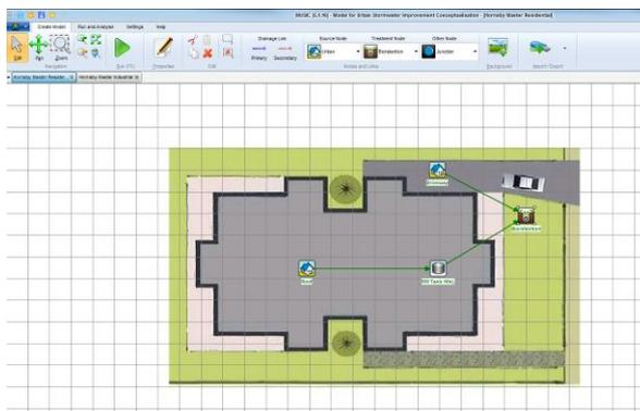
the pollution loads from the catchment. The bioretention system has an extended detention depth of 0.2m and a filter depth of 0.6m. The MUSIC modelling results are shown in the following table.
