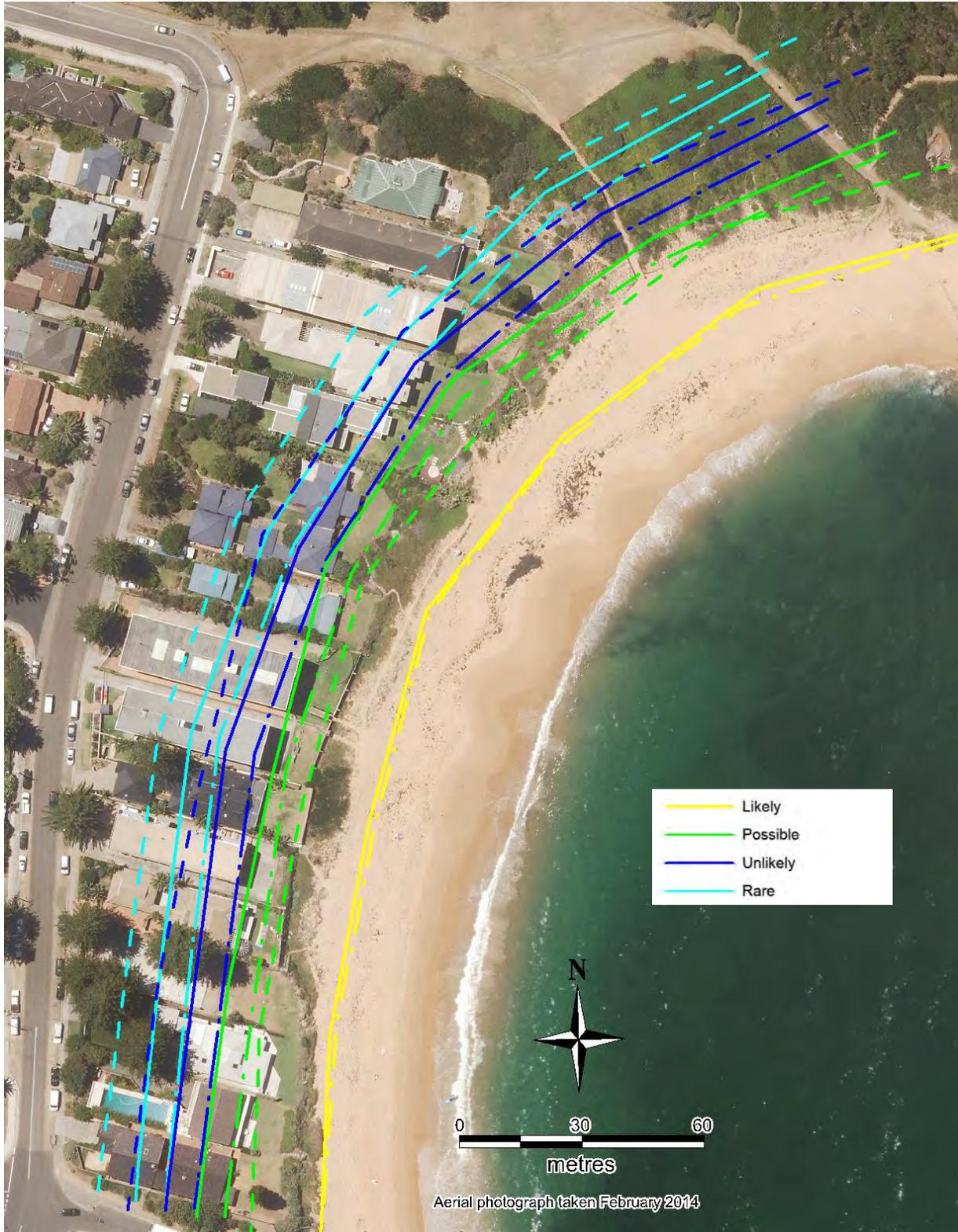
**Figure D10: 95% (dash dot line), 50% (solid line) and 5% (dashed line) exceedance recession scenario likelihood lines at Basin Beach for Type 2 procedure for 60 year design life (at 2075)**
