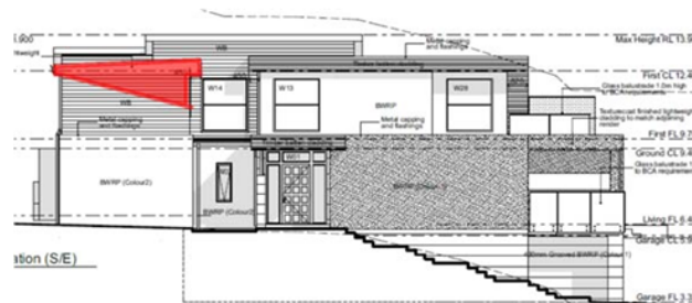
Figure 7: An extract of the southeast elevation; the approximate area of the envelope breach is highlighted in red.
