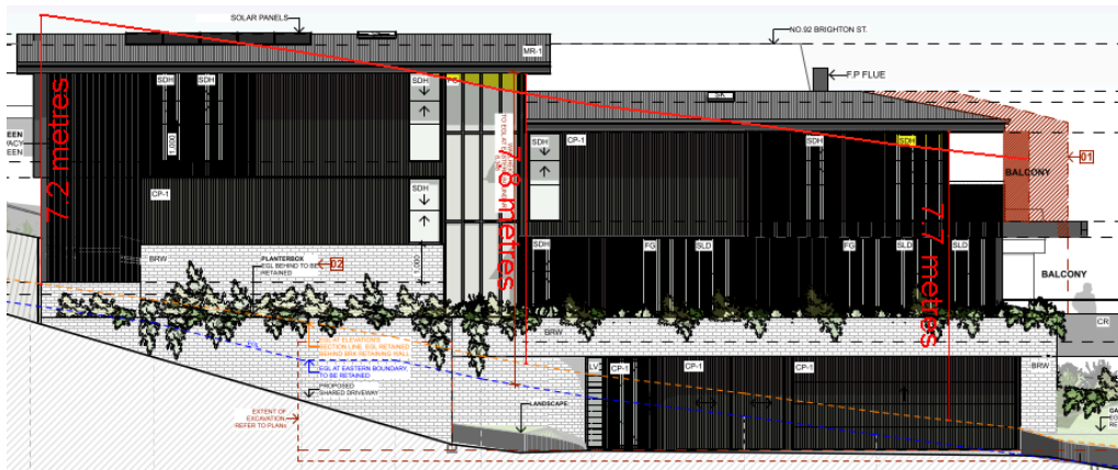
Figure 2 above: The wall height control line is depicted by the red line. The portions of the development breaching the wall height control on the eastern elevation of Lot 1, highlighted in yellow above the red line.
