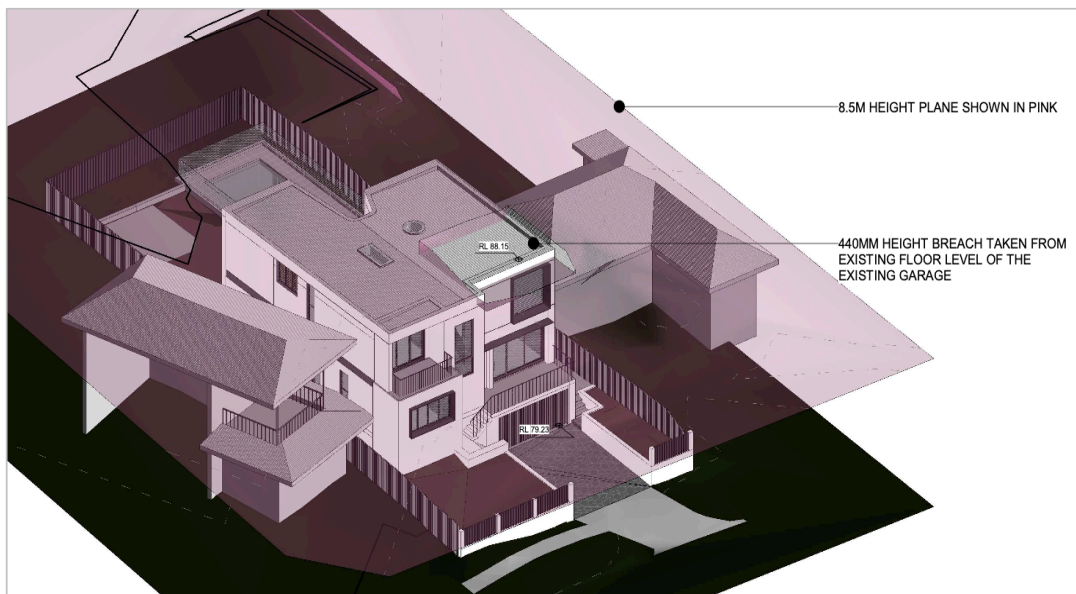
Figure 2: Height breach 3D diagram Source: HA S
