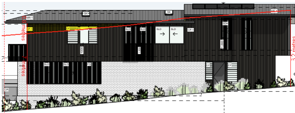
Figure 6 above: The side boundary envelope is depicted by the red line. The portions of the development breaching the envelope on the western elevation of Lot 2, highlighted in yellow above the red line.
