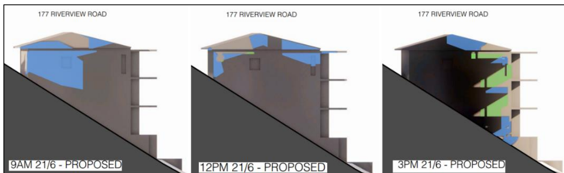
Figure 29 Shadow diagrams projected onto 177 Riverview Road at 9am, 12pm and 3pm on 21 June. Dark shadows indicate existing and continued overshadowing, blue indicates additional overshadowing from the proposal, green indicates reduced overshadowing from the proposal which presently exists from the existing dwelling house on site.
