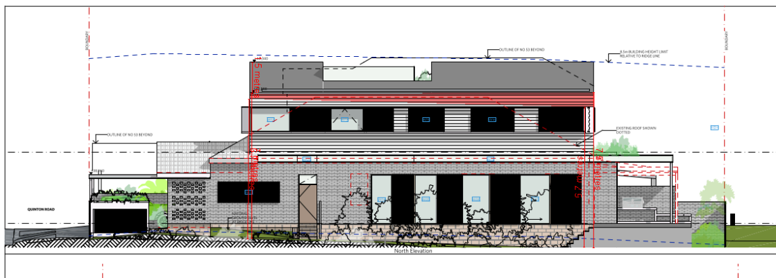
Figure 2: North elevation with wall height non-compliance shaded in red.
