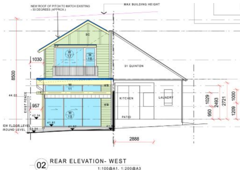
Figure 5: West elevation showing location of windows W17 and W18.
