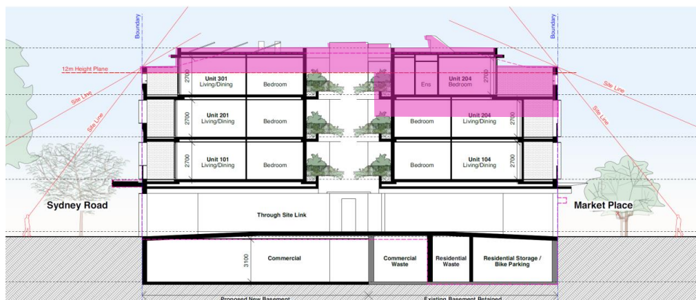
Figure 1: Extent of height breach when measured to existing ground levels
