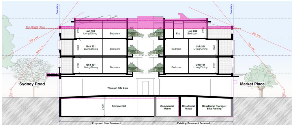
Figure 2: Extent of height breach when measured to finished ground levels
