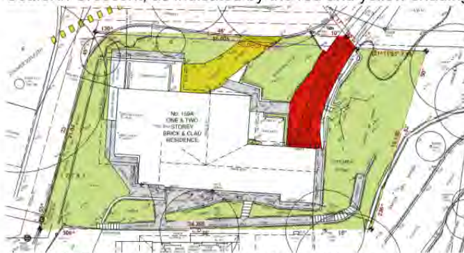
Figure 3. Existing driveways, indicated in yellow and red shading.
