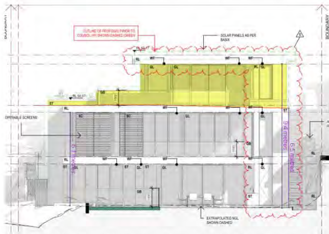
Figure 2. North-western elevation wall height non-compliance indicated in yellow shading.
