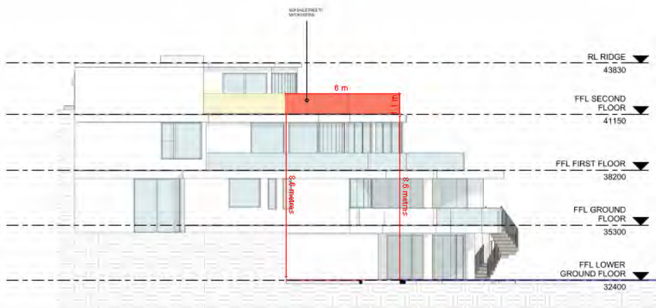
Figure 2 - East elevation showing envelope breach in red
