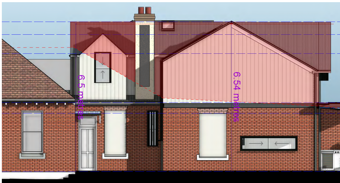
Figure 2. Southern elevation wall height non-compliance (extent shaded as red).
