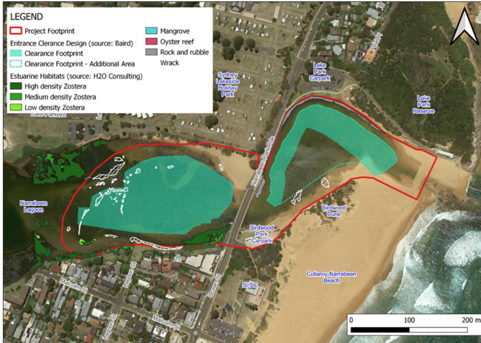
Figure 3-1: Entrance clearance works footprint
