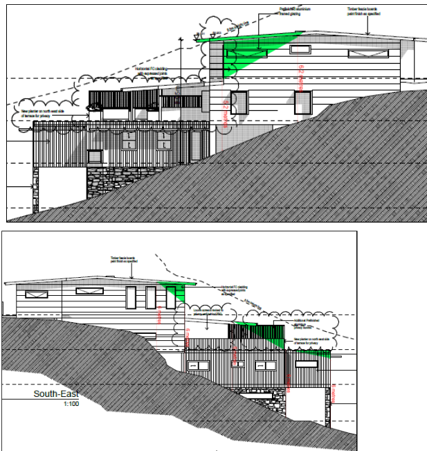
Image: SBE breach is largest at NW corner. This is due to angle boundary and topography.
