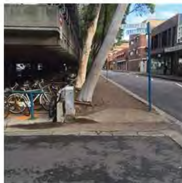
Dangerous crossing over the driveway exit from the car park; inappropriate kerb ramps; rubbish bins and bikes chained on poles often present in this area - obstructions and congestion on the main route to the library and Market Place.
