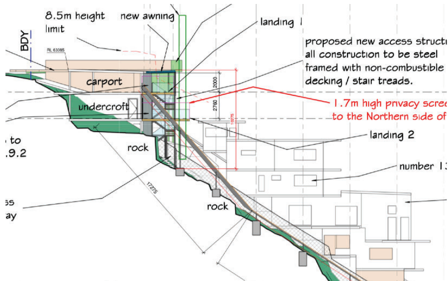
Figure 3: Plan showing height of awning over Landing No. 1, Source: Peter Downes Designs
