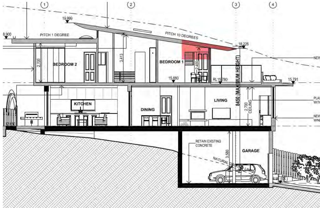
(Figure 1: Section 1 - Red shading to indicate building height non-compliance)
