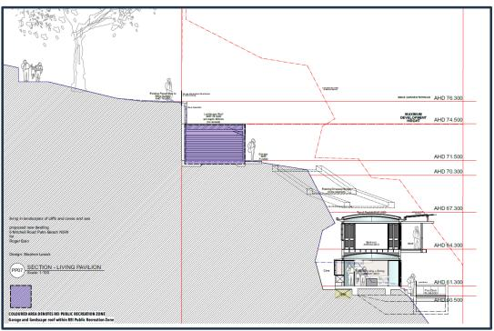
Figure 16: Concept Section detailing the garage as below the Bible Garden and height limit (Souce: Housed Architects)
