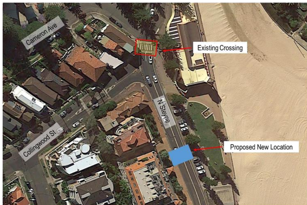
Figure 6.10: Concept Design Relocation of North Steyne Pedestrian Crossing
