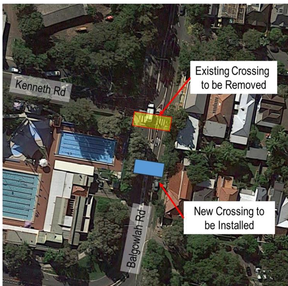
Figure 6.19: Option 2 Concept Design Relocation of Balgowlah Road Pedestrian Crossing
