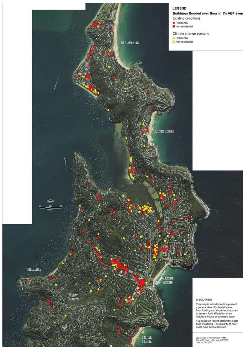
Figure 14.3 – Simulated changes in over floor flood affectation due to climate change
