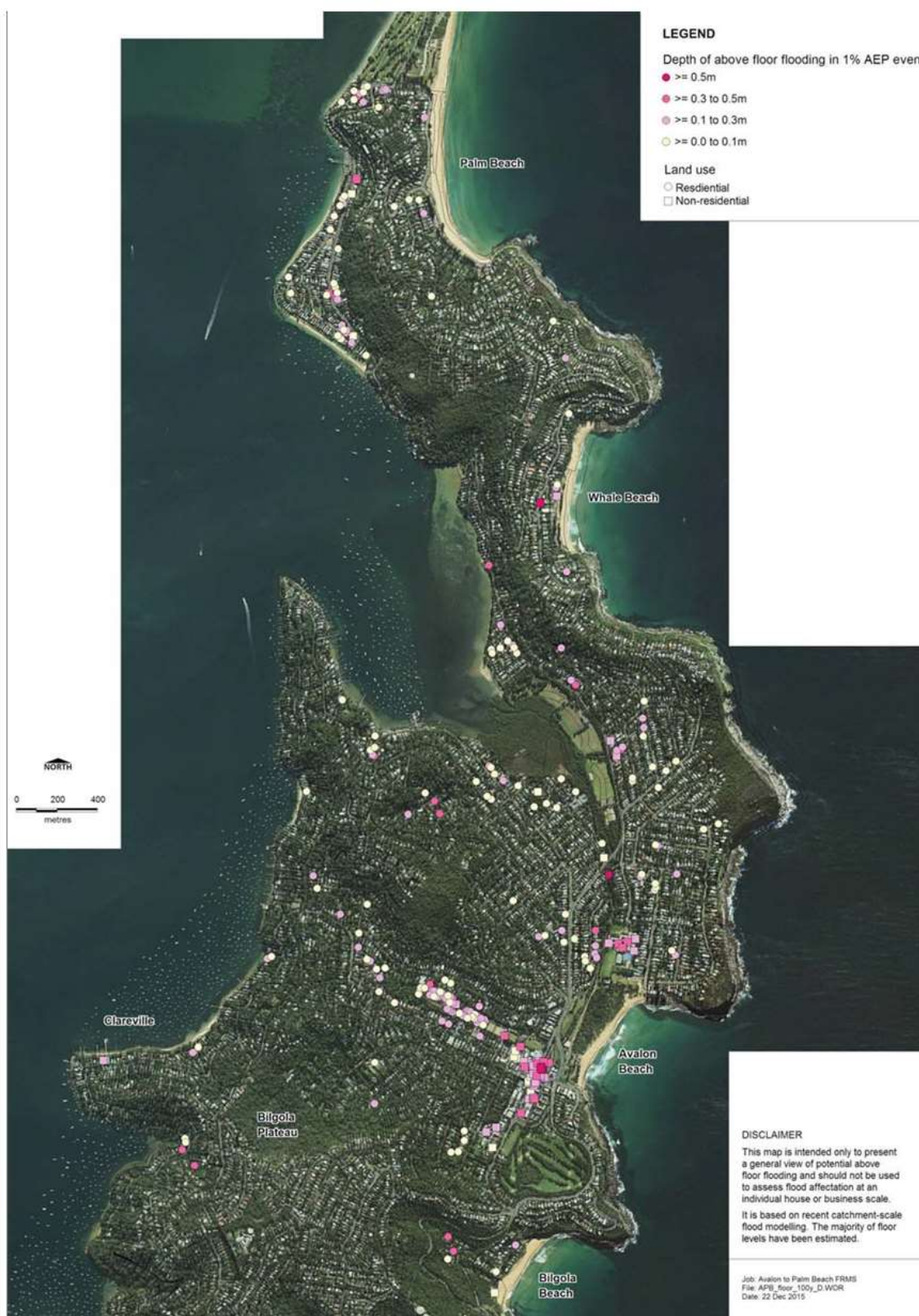
Figure 8.3 – Depth of above floor flooding in 1% AEP event
