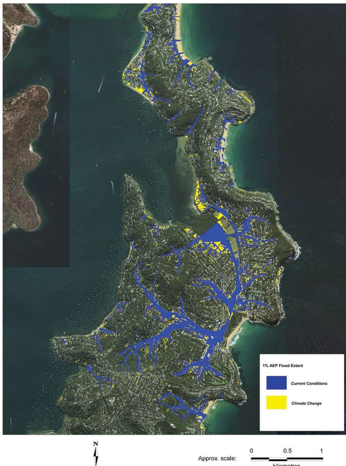
Figure 14.2 – Simulated changes in 1% AEP flood extent due to climate change
