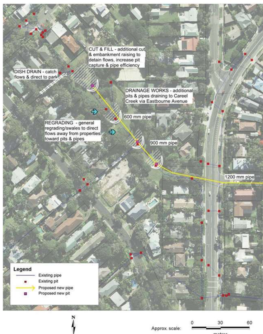
Figure 11.6 – Jamieson Park detention basin conceptual layout
