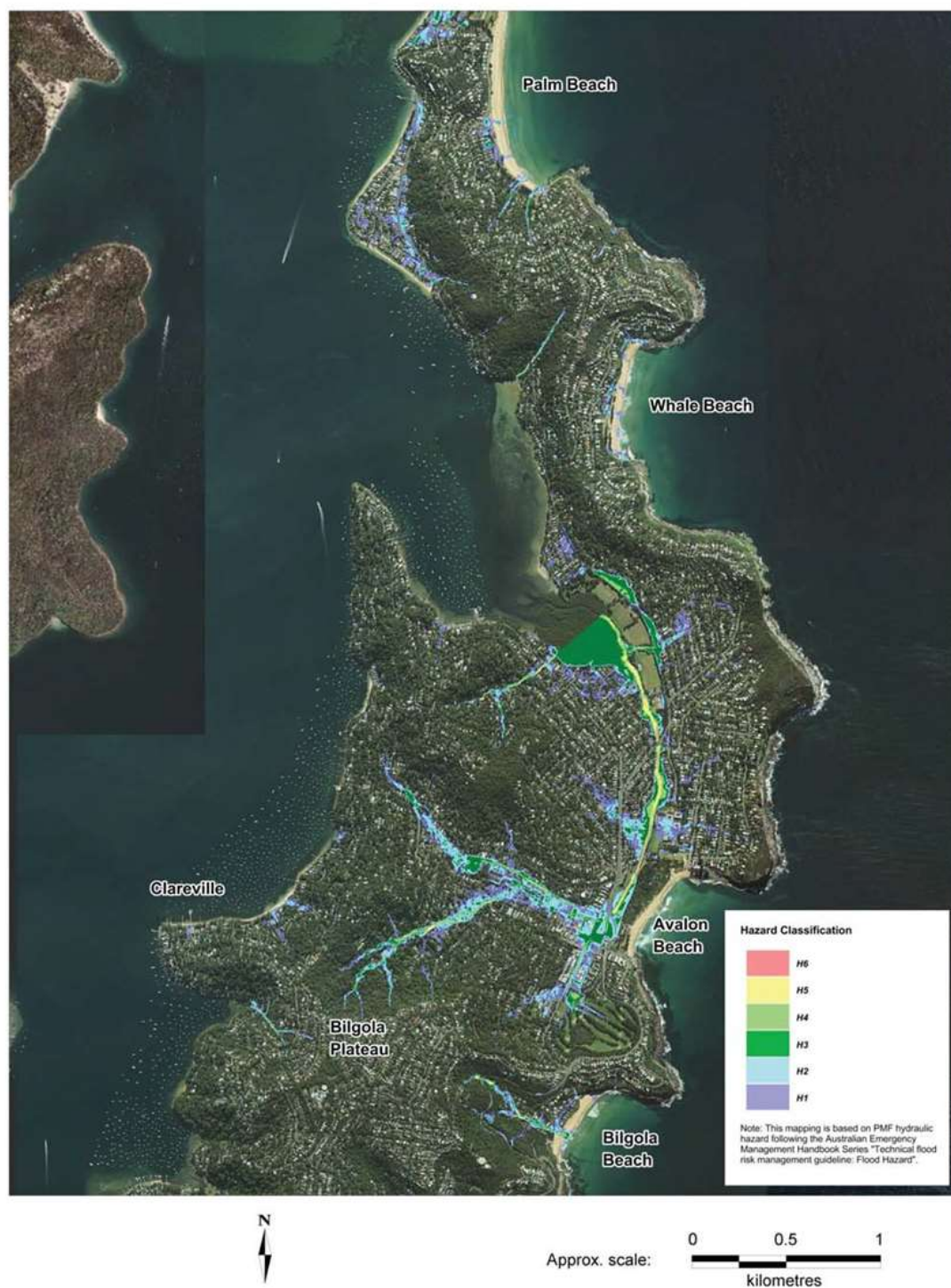
Figure 7.4 – Flood hazard in the 1% AEP
