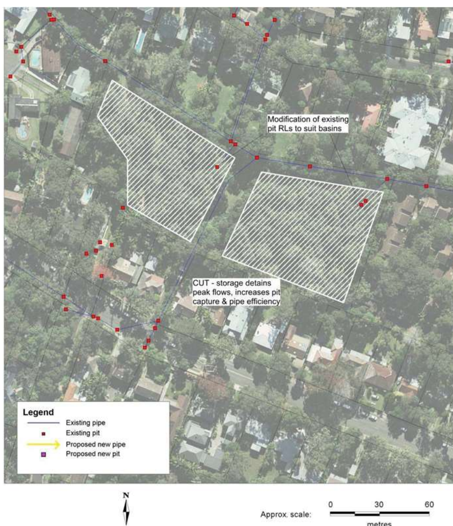
Figure 11.4 – Toongarri Reserve detention basin conceptual layout
