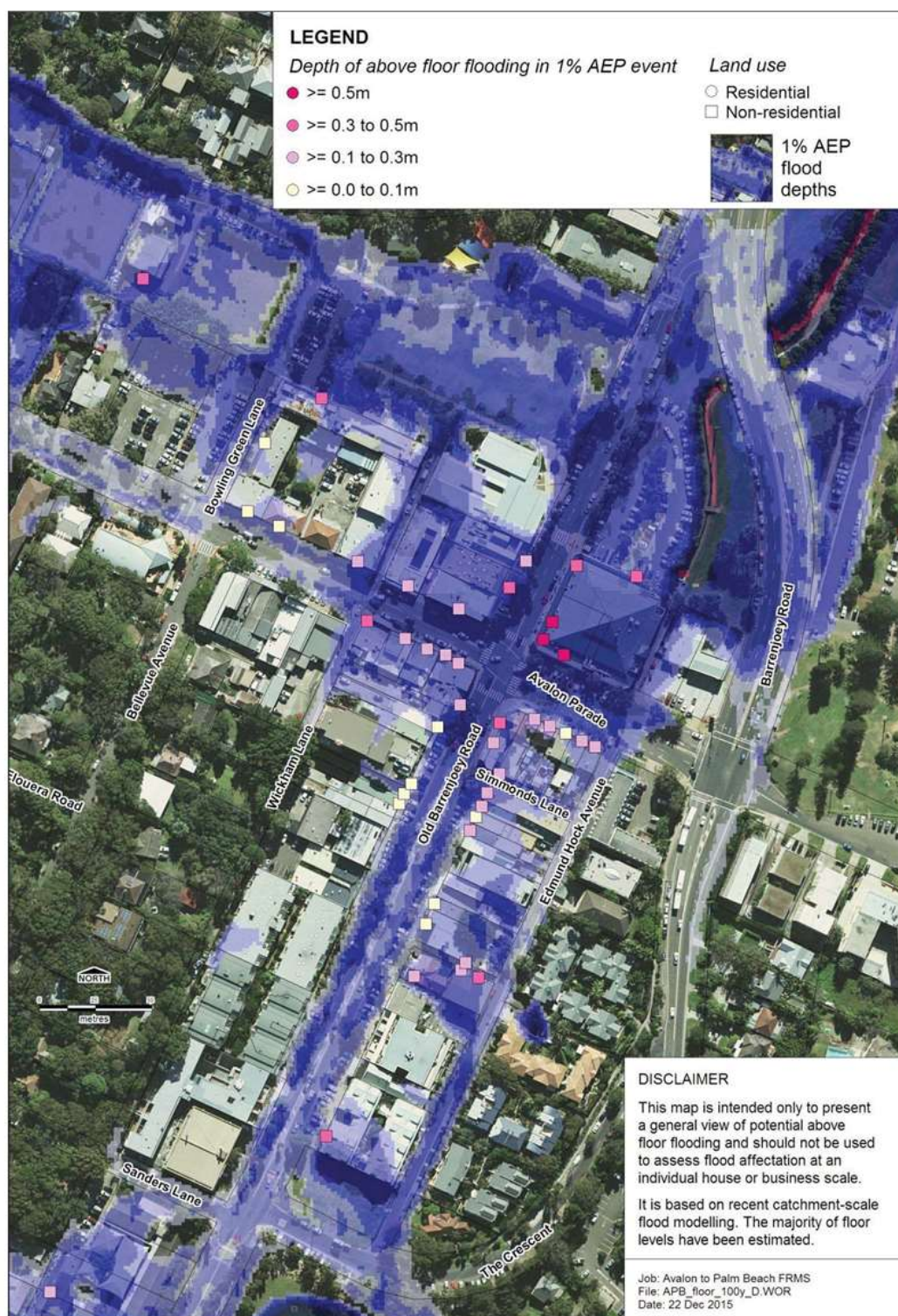
Figure 8.5 – Depth of above floor flooding in 1% AEP event, Avalon shopping centre
