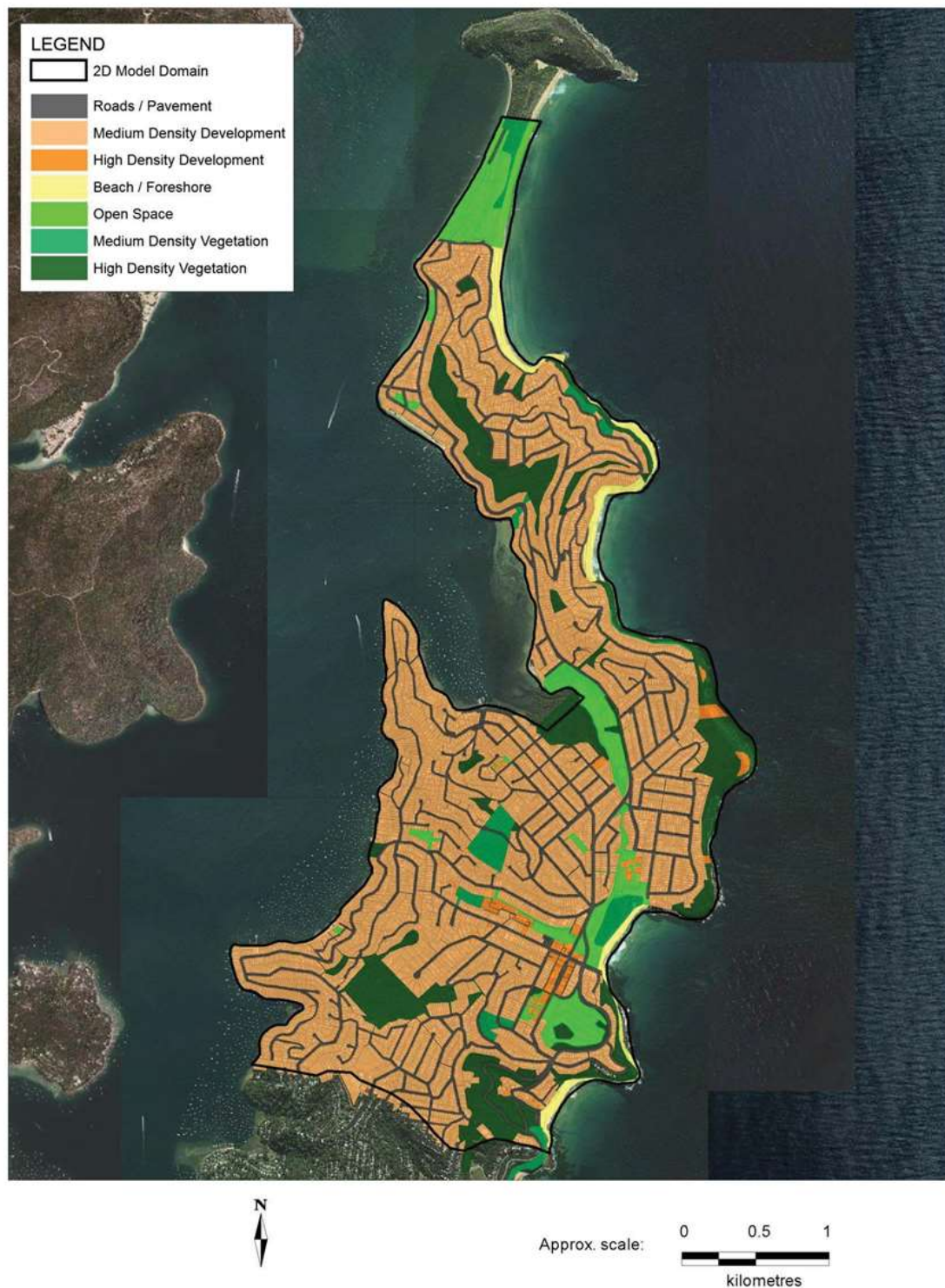
Figure B2 Hydraulic Roughness Zones
