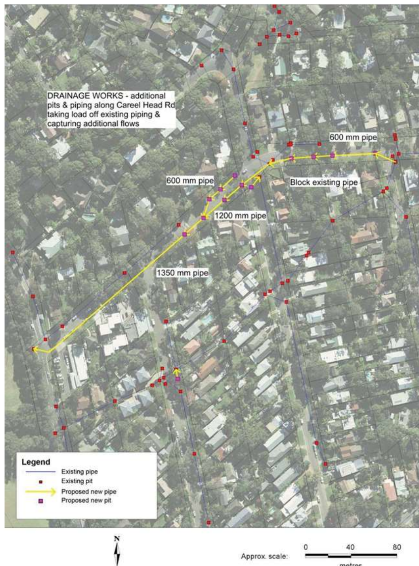
Figure 11.7 – Careel Head Road drainage upgrade conceptual layout
