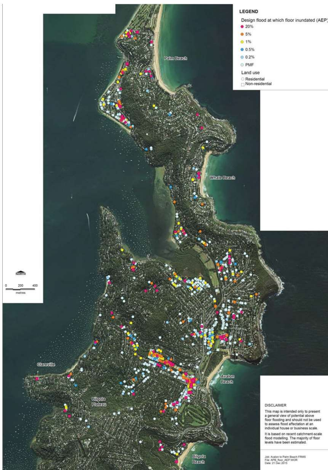
Figure 8.2 – Buildings flooded over floor by design event
