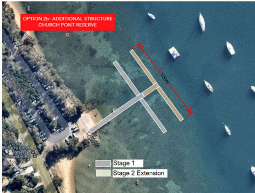
Figure 3-5 Option 2b Staged Concept Floating Pontoons Church Point Reserve. Stage 1 Additional 90 Boat Bays and Stage 2 Additional 90 Bays.
