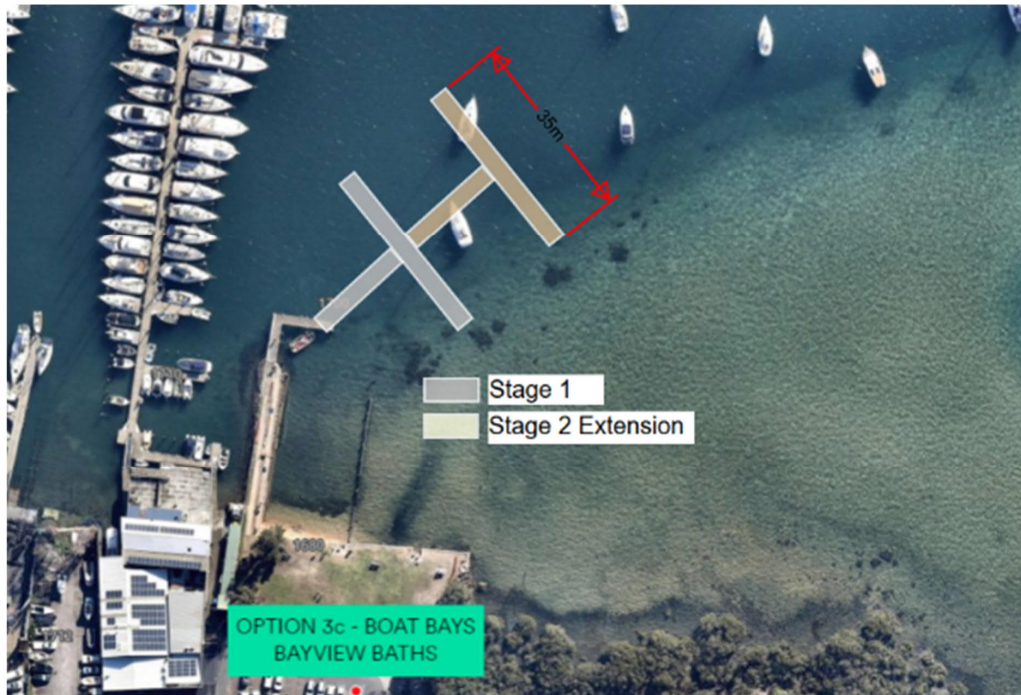
Figure 3-10 Option 3c Concept Floating Pontoon Bayview Baths. Stage 1 Comprises an Additional 32 Boat Bays. Stage 2 Additional 32 Boat Bays. Total Increase in Berths 64.
