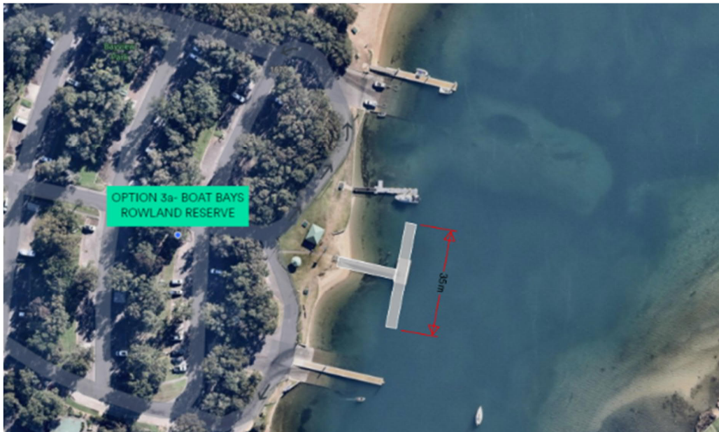
Figure 3-8 Option 3a Concept Floating Pontoon Rowland Reserve. Additional 32 Boat Bays.
