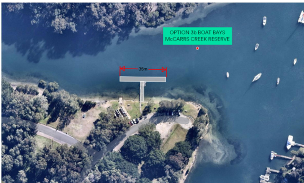
Figure 3-9 Option 3b Concept Floating Pontoon McCarrs Creek Reserve. Additional 32 Boat Bays.
