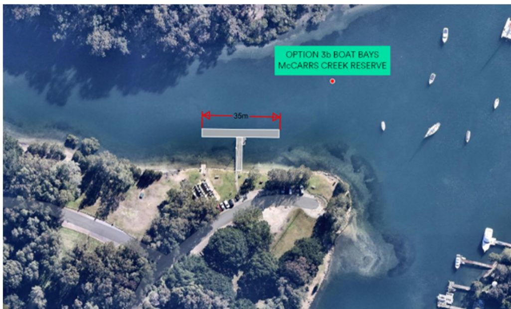
Figure 5-11 Option 3b Concept Floating Pontoon McCarrs Creek Reserve. Additional 32 Boat Bays.
