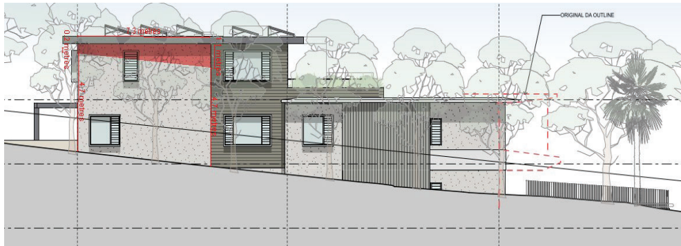
North Elevation envelope breach (source Gartner Trovato)
