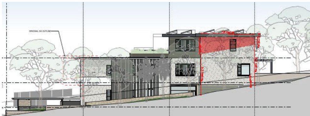
South Elevation envelope breach (source Gartner Trovato)
