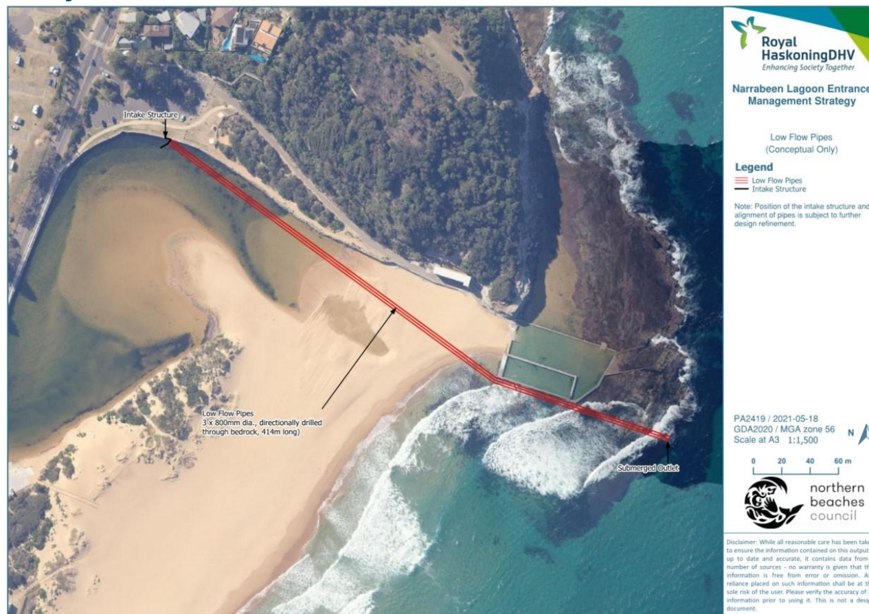
Figure 6-7: Low flow pipes option conceptual arrangement
