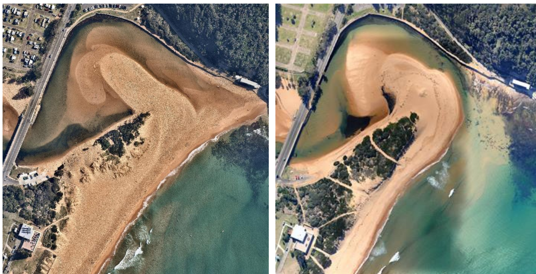
Figure 2-9: North Narrabeen beach states (Left: October 2020 – clockwise rotation; Right: June 2010 – anti-clockwise rotation)
