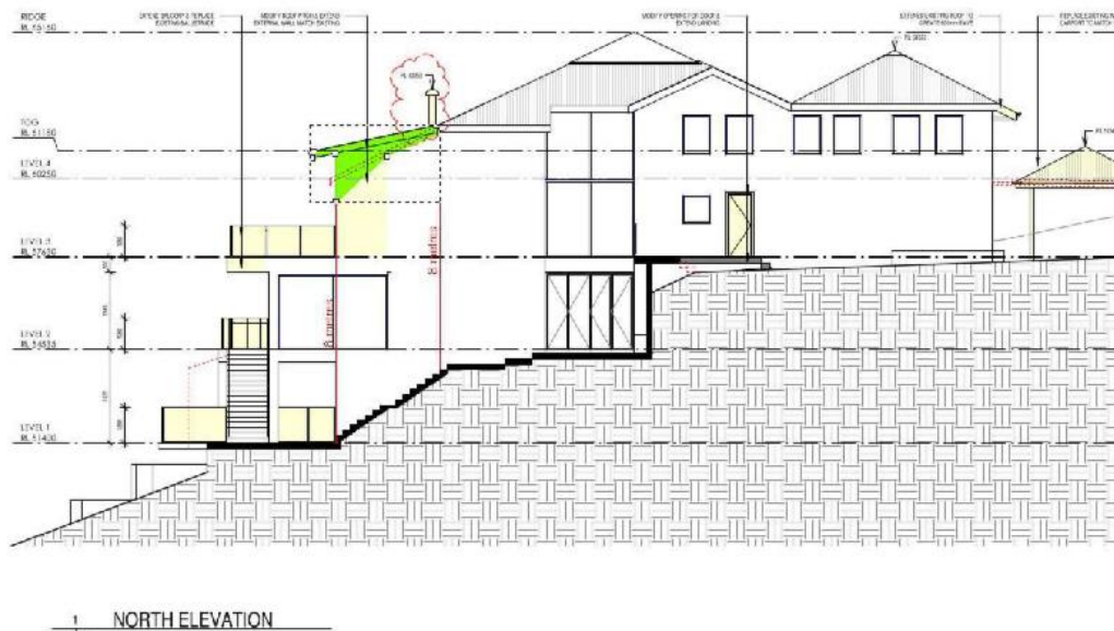
Figure 2: Building height non-compliance of proposed works shown in green (North Elevation)
