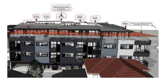
**Figure 2** - Plan extract DA041(E) showing the building height breaching elements proposed above the 11 metre building height standard as viewed from Somerville Place
