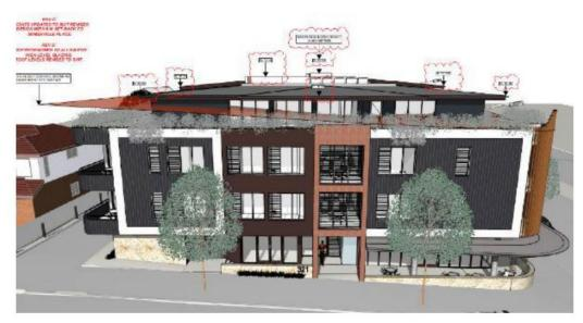
**Figure 3** - Plan extract DA042(E) showing the building height breaching elements proposed above the 11 metre building height standard as viewed from Sunshine Street
