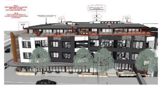
**Figure 4** - Plan extract DA043(E) showing the building height breaching elements proposed above the 11 metre building height standard as viewed from Condamine Street
