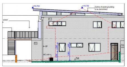
Figure 2: Proposed building will position brick side wall toward rear of existing eave as shown in the elevation overlay.
