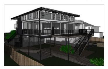
Figure 1: Perspective view showing operable glazing and view line.
