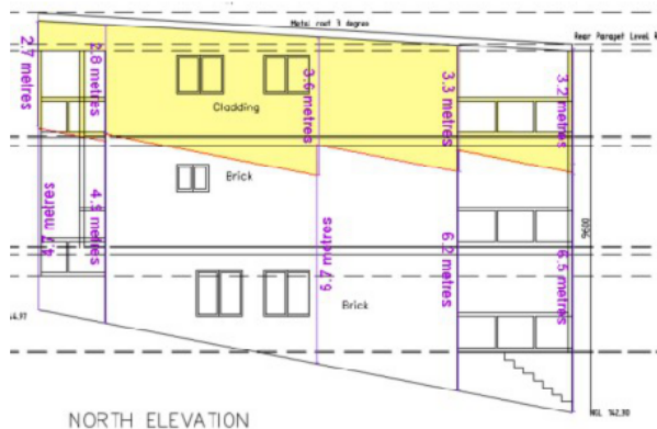
Image 1. North Elevation envelope breach (in yellow).
