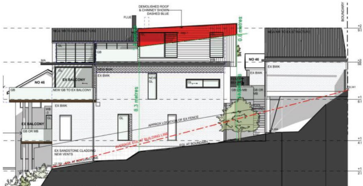
Figure 2: Eastern Building Envelope Variation Source: Annotated Architectural Plans, Watershed Design DA13 Issue G
