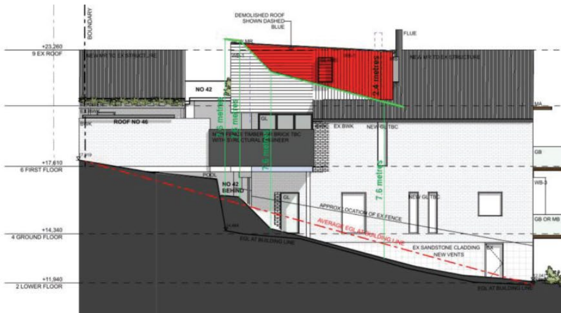
Figure 3: Western Building Envelope Variation Source: Annotated Architectural Plans, Watershed Design DA14 Issue G
