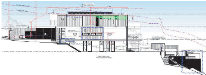
Figure 2: Southern elevation wall height non-compliance shown in green.
