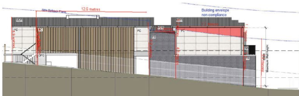
Side Boundary envelope breach - west elevation.
