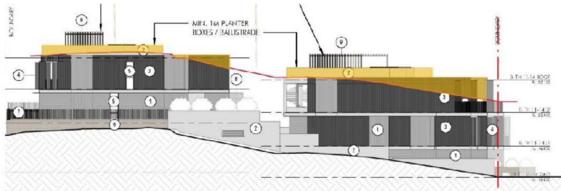
Figure 3: Western Elevation - Non-compliance with Side Boundary Envelope, shown in yellow (source: Statement of Environment Effects by Symonds Goodyer).
