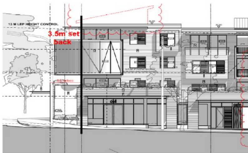
Elements that breach the 3.5m and 6m set back to intersection of Waratah Street and Bungan Street.
