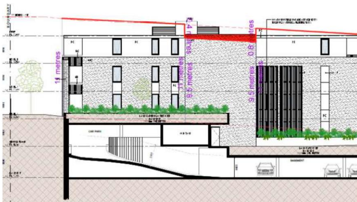
Figure 2: Eastern Elevation - Non-compliance with Side Boundary Envelope shown in red
