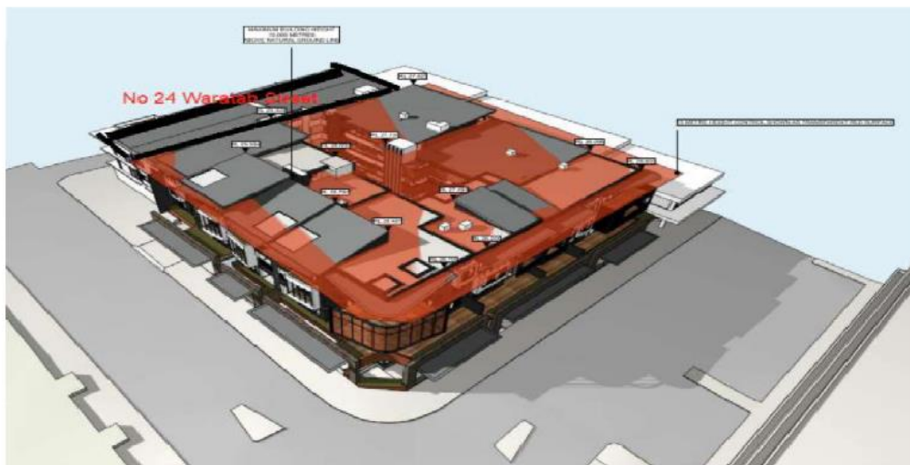
Height control image illustrating the non compliant roof projections and lift overrun above the 13m height limit.
