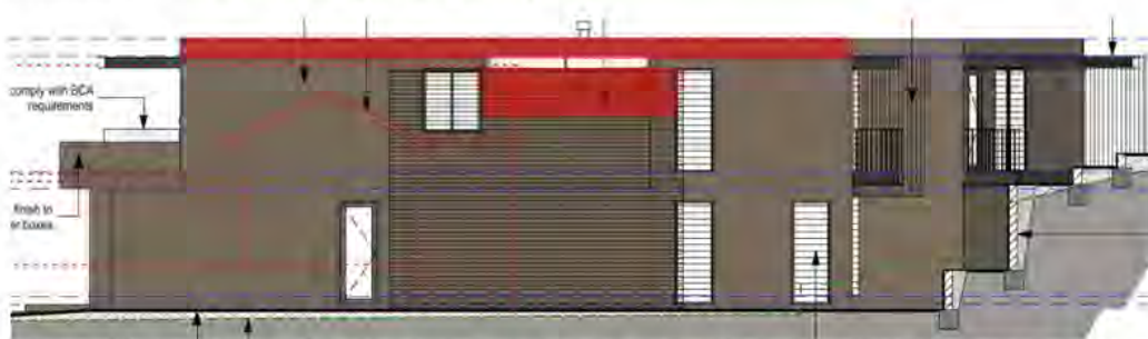
Figure 23: An extract of the proposed northern elevation of the dwelling; the breaches of the building envelope are indicated by the red boxes.
