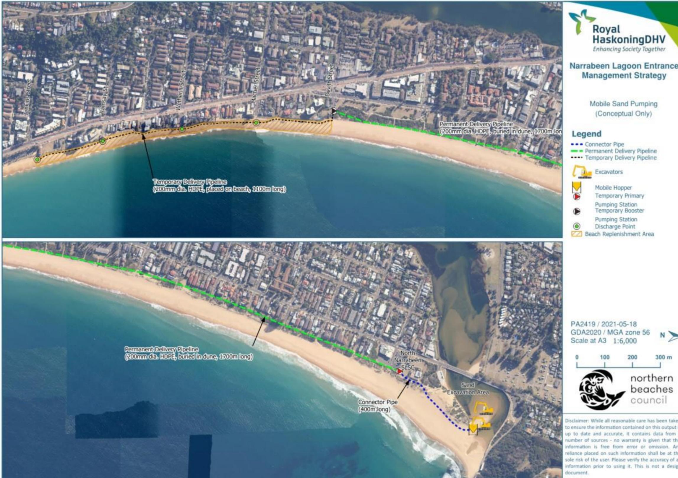
Figure 6-4: Mobile sand pumping option conceptual arrangement
