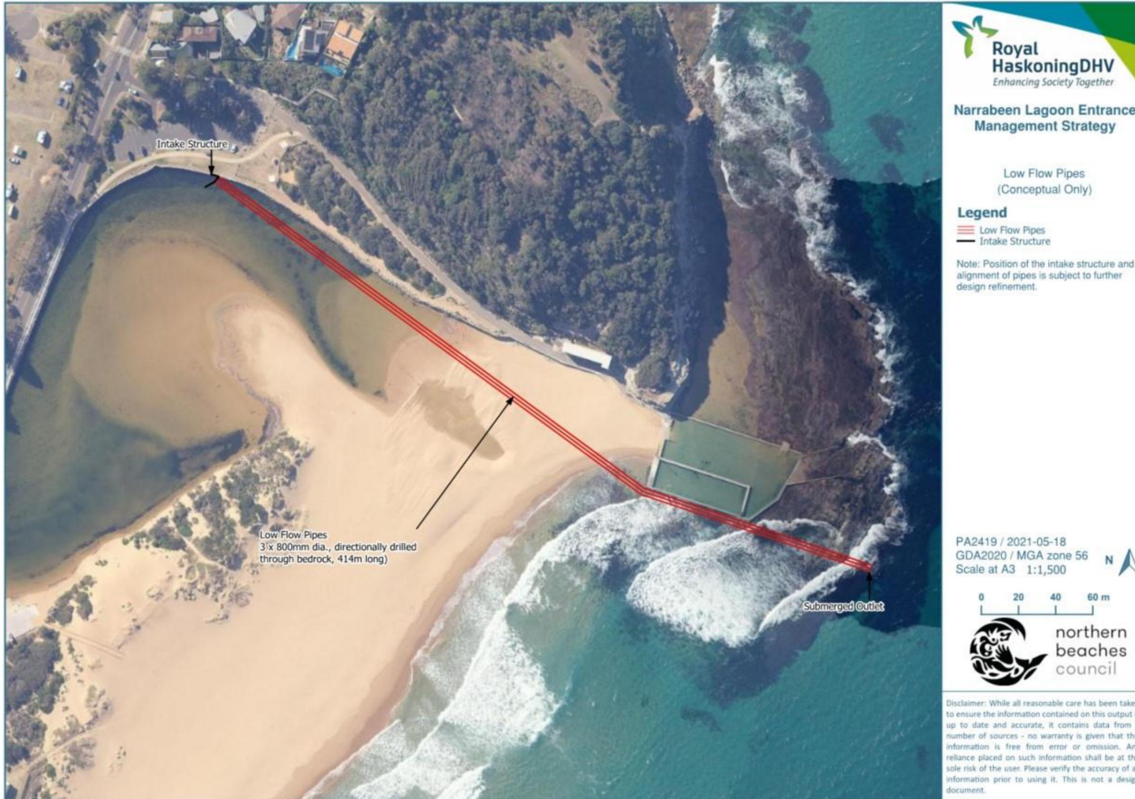
Figure 6-7: Low flow pipes option conceptual arrangement
